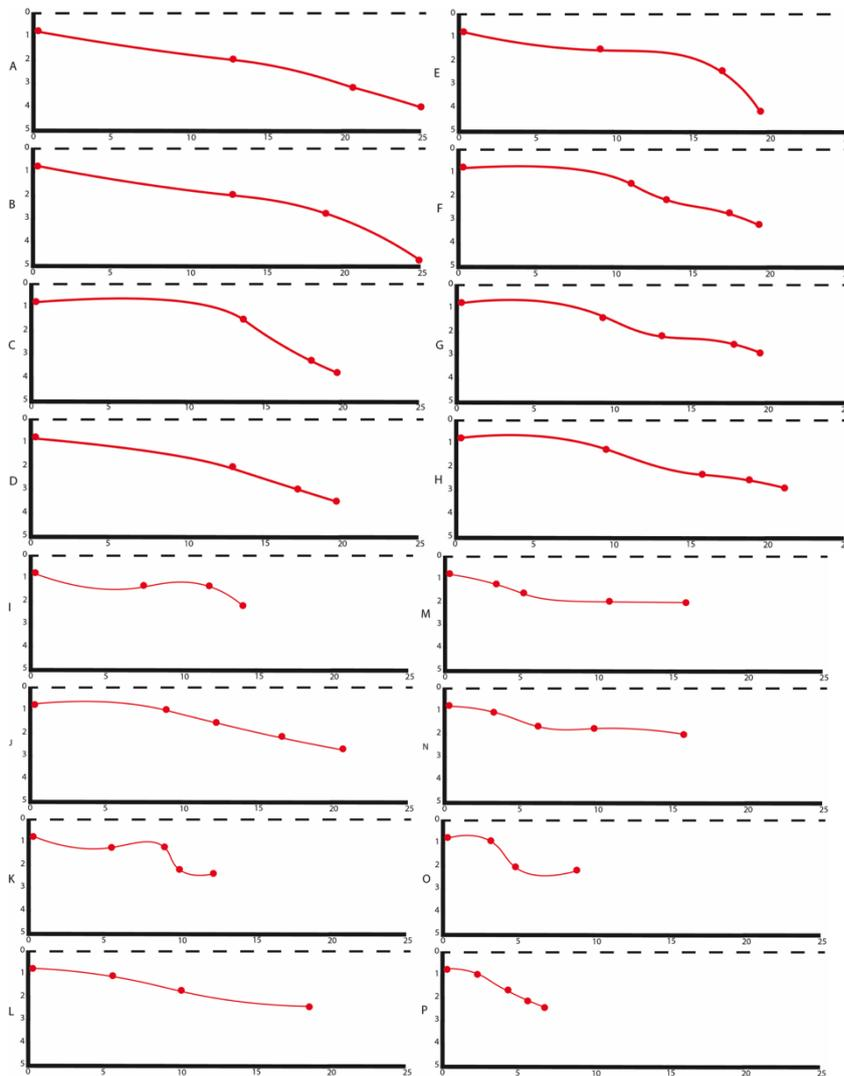
Figure 11. Profiles from south to north (A-P) along the eastern edge of the breakwater to the north-eastern extent of the rubble (M. Polidorou)
