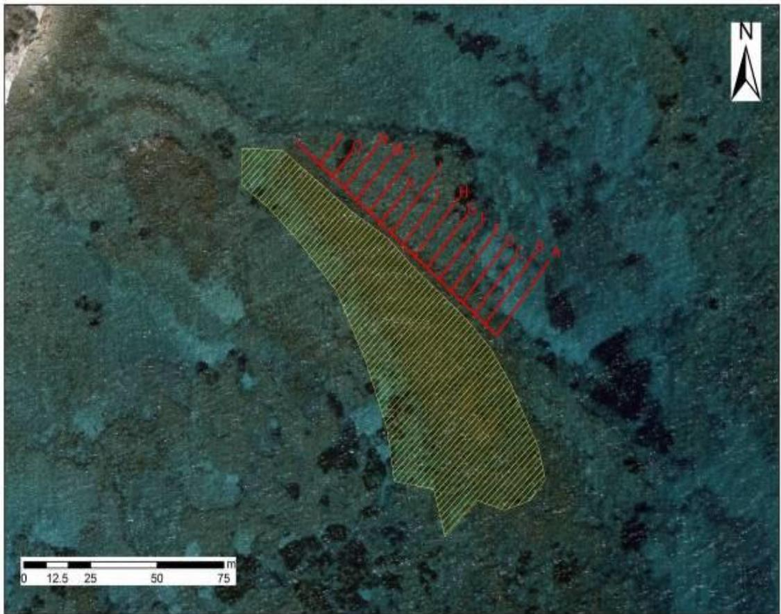
*Figure 10: Maximum distances (ref to Table 1) of rubble east of the breakwater. NB. The yellow lines identify the area of the breakwater. The red line that runs along the eastern edge of the breakwater indicates the position of the baseline tape and the survey lines that extend perpendicular out from this towards the northeast, to the maximum extent of the rubble (M. Polidorou).*
