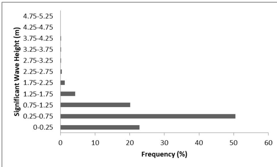
Figure 12: Frequency of Significant wave Height (m) measured at the study area between 1961-1990 (Loizidou and Dekker 1994)
