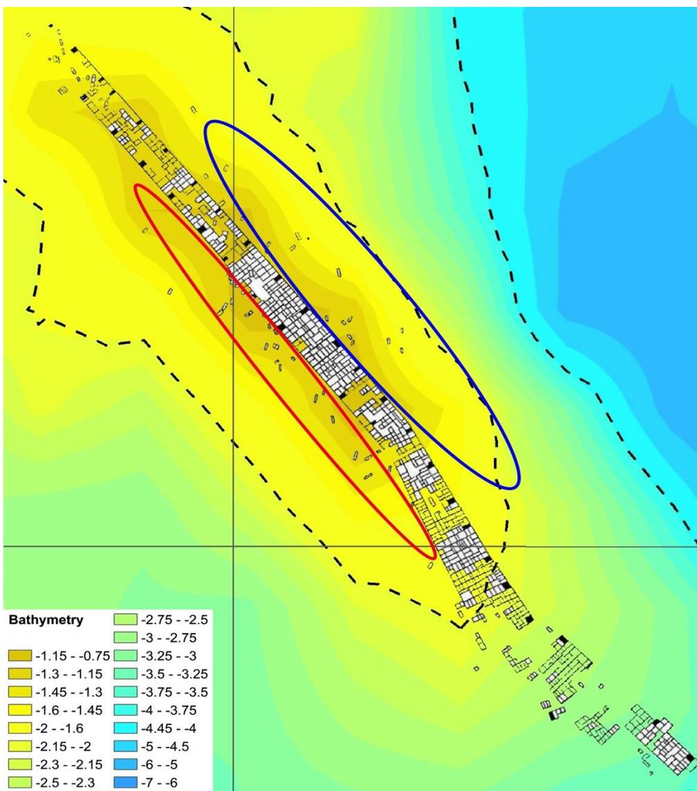
Figure 9: Schematic representation of the rubble orientation either side of the breakwater (M. Polidorou).
