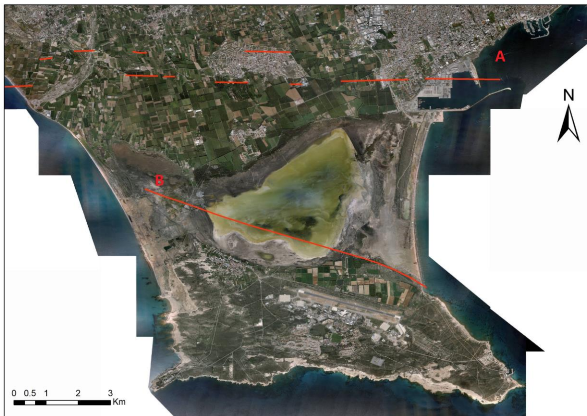
Figure 10: Active Quaternary Faults. A. Left-lateral strike-slip faults with vertical component orientated E-W, B. Strike- slip fault with vertical component orientated NW-SE (Geoter, 2003)
