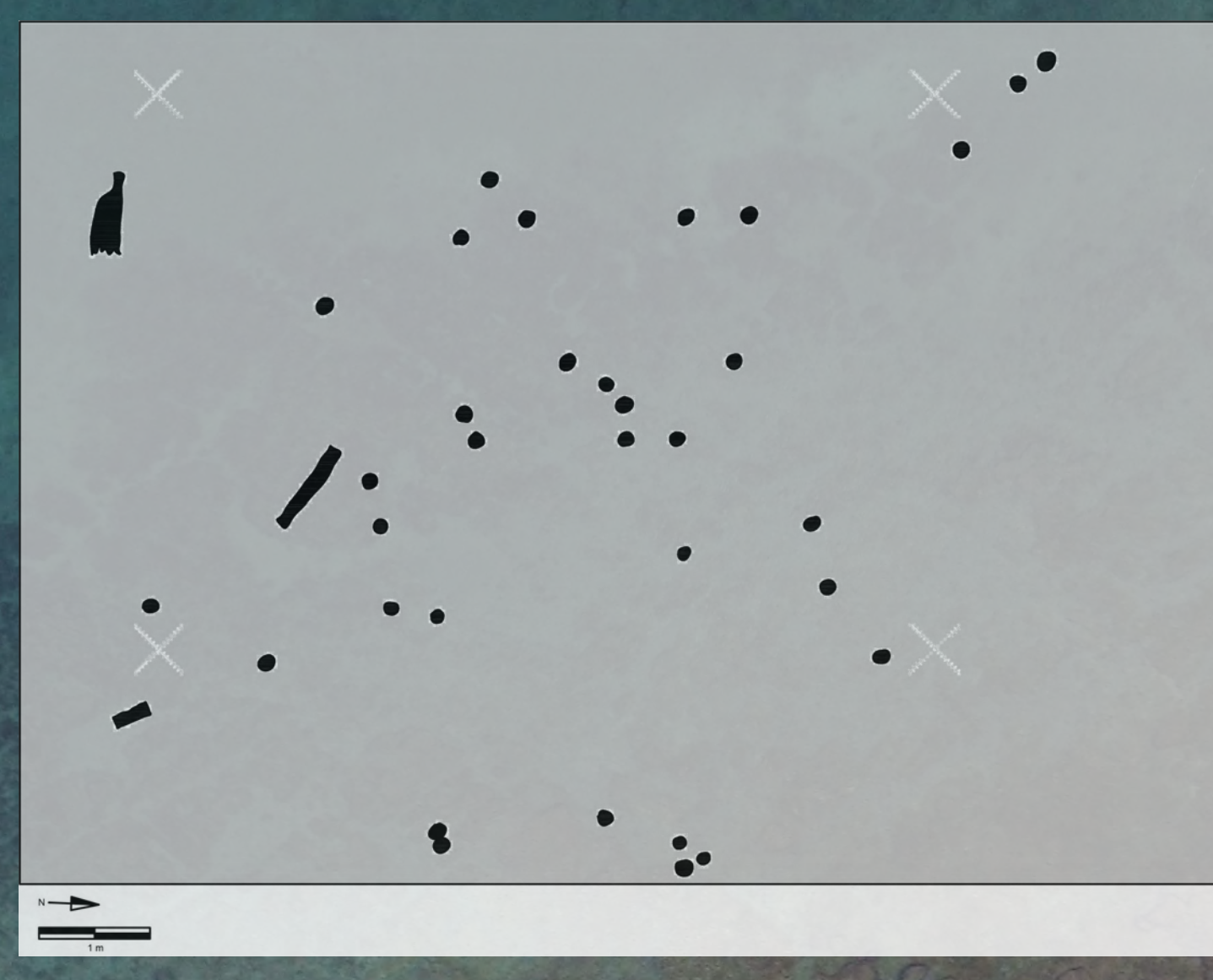
Figure 8: Drawing of a small section of the site. The black dots represent wooden piles. Author: I. Koncani Uhac 2017, modified by K. Jerbic.
