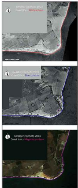
Fig.4: Orthophotos 1963, 1993 & 2014. The layering of the shoreline has been drawn for three different periods (1963 in red, 1993 in blue, 2014 in magenta) (Department of Lands and Surveys)
