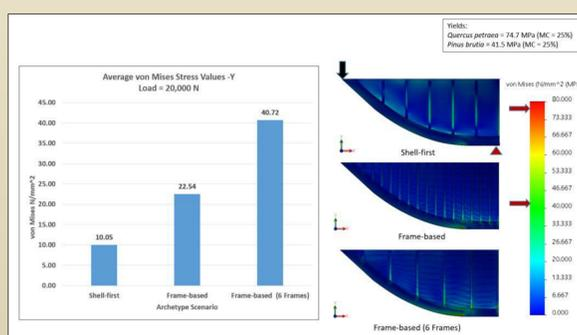
Figure 7: Archetypal von Mises stress results.
