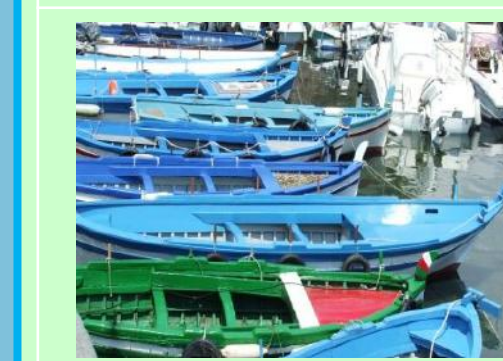
Fig. 10. Boats crowded in Ognina. There were over 100 boats all of which appeared to be regularly maintained and many put to sea providing fish for the family. They are very important status symbol amongst the male population. Many of them are canoe stern and are propelled by oars or outboards fitted to a small wooden bracket. Note the range of different stem extension shapes. These are used as identifiers between the local fishing communities and it is apparent that a collection of boats from along the coast has accumulated here. The strong association with the sea perhaps dates back to the time of the Phoenicians. The relatively high abundance of fish in the local waters may have maintained the traditions, whereas declining fish stocks accompanied the decline in traditional boats and boat building.
