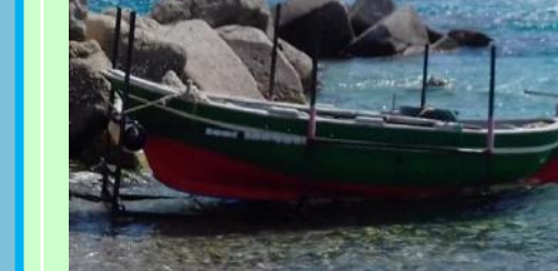
Fig. 12. A Messina fishing boat. The curved, flared bow is the main difference in design compared to the other boats along this coast. They are launched and recovered using a specially built wheeled trailer, that would appear to be unique to the beaches close to Messina. There are two distinct colour schemes with which the boats are decorated to distinguish them from one of two beaches. Today they mostly have an inboard engine and rudder, but in the past sails and more commonly oars would have propelled these boats.
