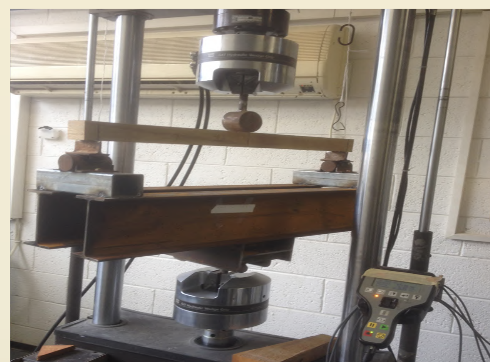
Fig. 4: Set-up of a beam bending test (According to ASTM D143-4)
