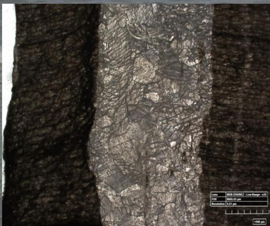
Fig. 2. Thin section of a rock, showing calcite vein and layers of clay minerals. Photo: H. Kravits, by 3D digital (HIROX RH-2000) microscope
