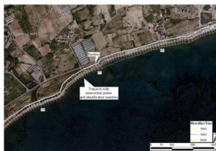
Left: Transects perpendicular to the 1963, 1993 and 2008 coastlines (produced in DSAS based on data provide by the Dept. of Lands and Surveys). Right: Net shoreline analysis movement. The results are visualised in different colours. Red indicates areas that are experiencing the highest rates of coastal erosion.
