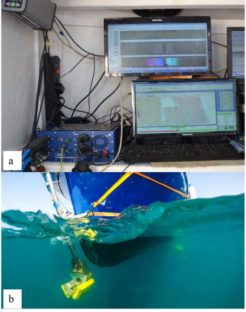
*Fig. 3.2.1.* The digital recording unit (a) and the transducers (b) of the ITER Systems BathySwath1 interferometric multibeam echosounder.
