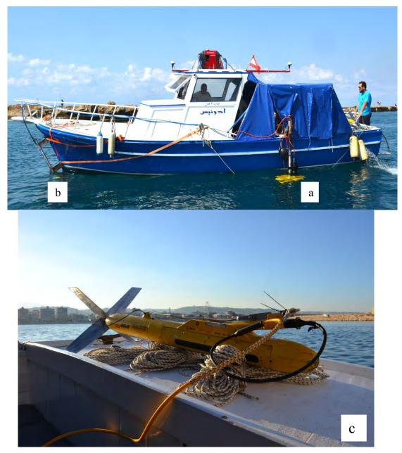
**Fig. 3.1.** The vessel "Adonis" which was used for the survey equipped with (a) the subbottom profiler (over-the-side), (b) the interferometric multibeam echosounder and (c) the side scan sonar system.
