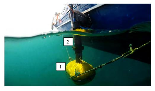
*Fig.3.1.1.* O.R.E. Model 138C over-the-side Transducer Mounting (1) and waterproof digital profiler electronics bottle (2).
