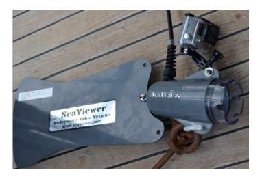
Fig.5. 1. The Sea Viewer underwater towed camera
