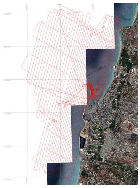
**Fig.3.2.** Map of the survey area showing the ITER Systems BathySwath1 interferometric multi beam echosounder, Chirp subbottom profiler and SideScan Sonar survey tracklines.
