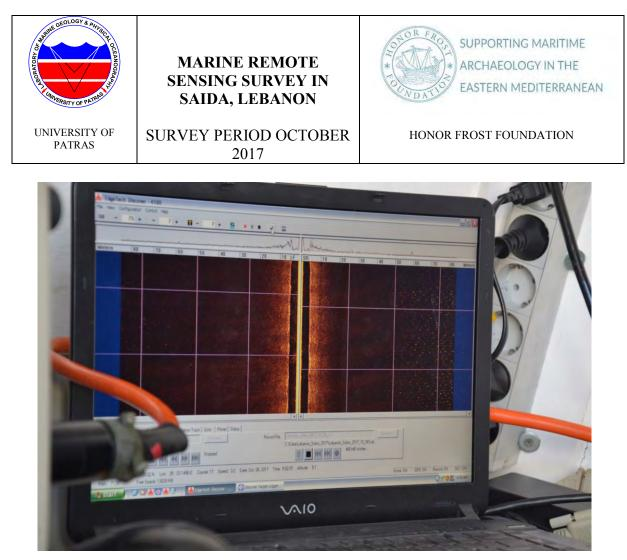
Fig.3.3.2. The Side Scan Sonar digital recording unit.
