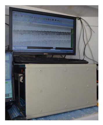
Fig. 3.1.2. GEOPULSE model 5430P digital recording station.
